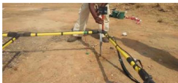
Figures 27 and 28: Example - Detector confirmation test using target (FFE) and detector manufacturer's test piece and ruler (Photos provided by Doug Ware, UNMAS)
