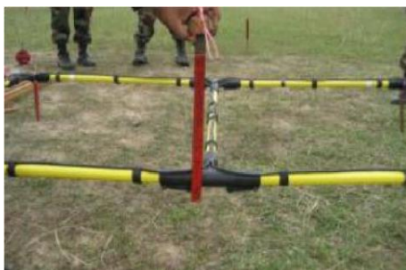
Figures 27 and 28: Example - Detector confirmation test using target (FFE) and detector manufacturer's test piece and ruler (Photos provided by Doug Ware, UNMAS)
